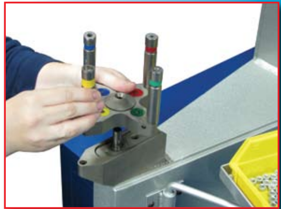
Turret easily removed and reinstalled with no realignment needed.
