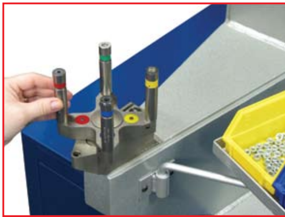
Turret easily rotated by hand.
